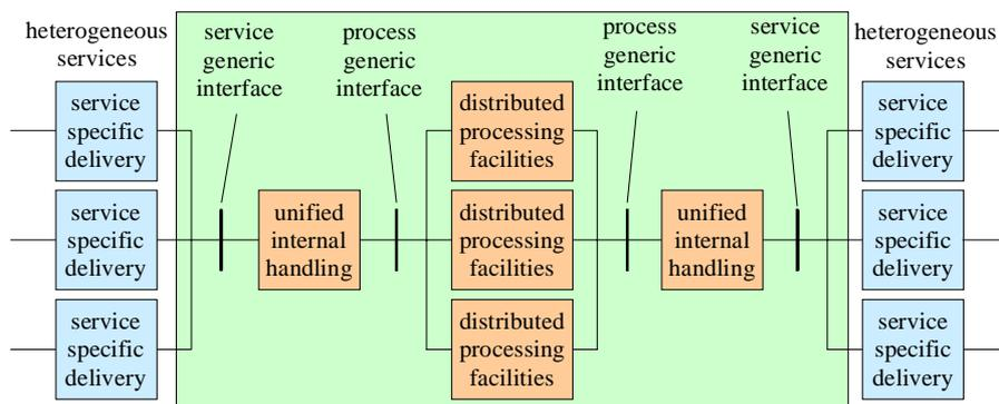
Figure 3: Generic interfaces for heterogeneous external services and internal components
