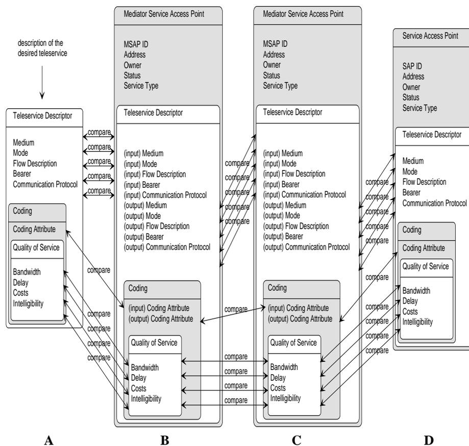
Fig. 2. Dynamic Resource Selection – Converter Chain containing TSD, MSAP, SAP attributes to terminals and converters, so that the input and/or output of a terminal or converter could be described in a generic way.
