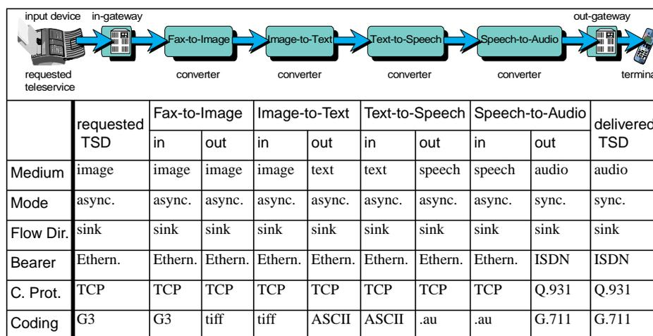
Fig. 6. Dynamic Resource Selection – Converter Chain with TSD mappings
