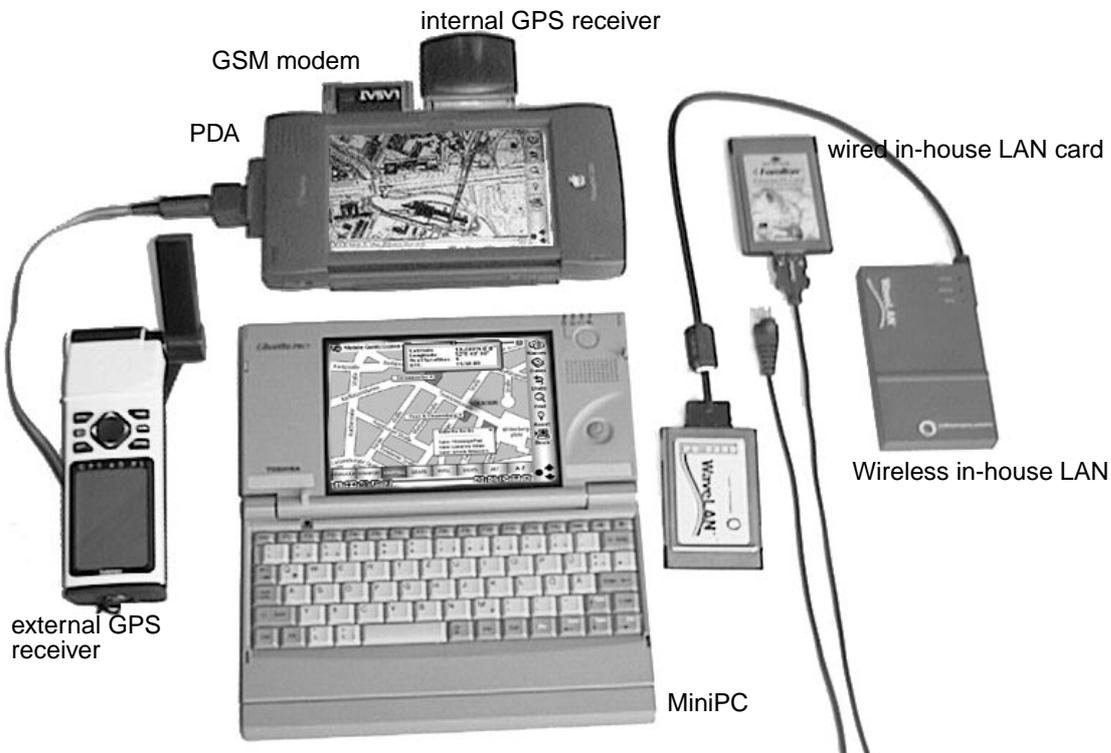
**Figure 8 Compact PDA with integrated, exchangeable positioning and communication technology**
