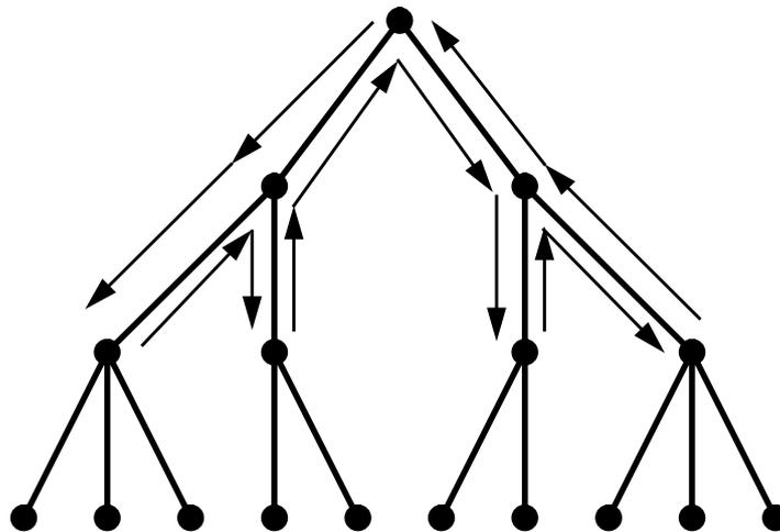
FIGURE 6 Virtual loop in a treelike distribution topology
