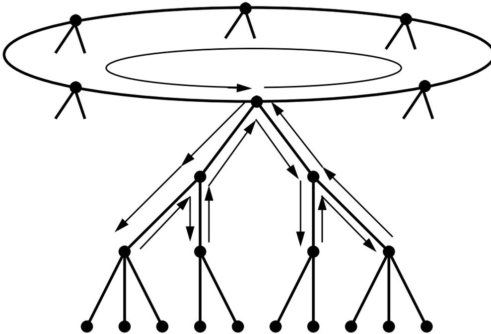
FIGURE 7 Virtual loop with a backbone ring topology
