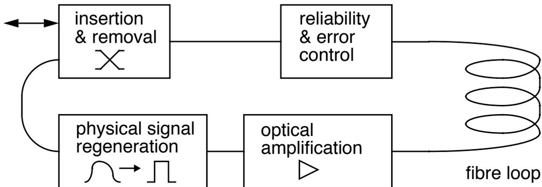
FIGURE 2 Functional elements of optical latency storage
