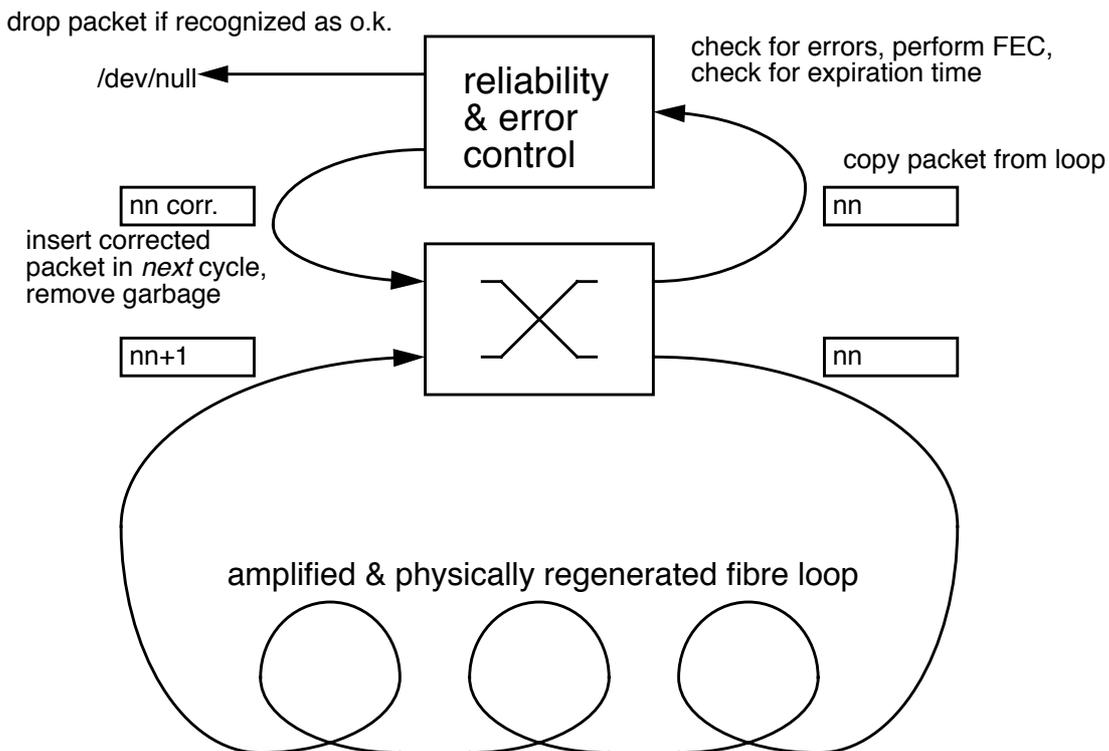
FIGURE 4 Error control with on-the-fly repair and next-cycle replacement
