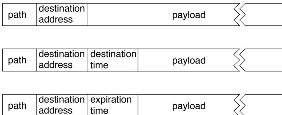
FIGURE 8 Packet headers for routing through space and time
