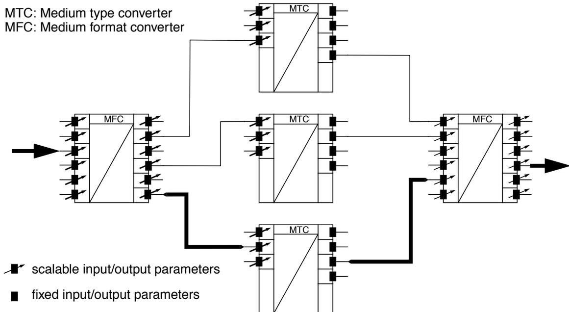
FIGURE 5 Medium type conversion with format adaptation
