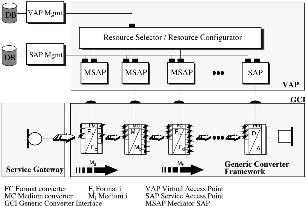
FIGURE 6 Dynamic Interworking of Converter Elements
